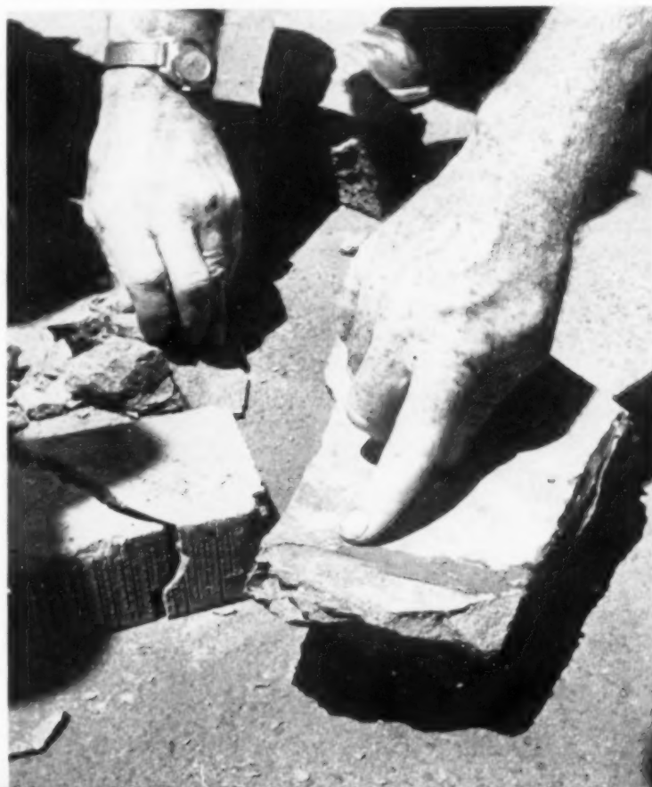
In test, brick breaks before joint
